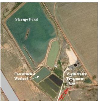
Figure 1: Junee Wastewater Treatment Plant
